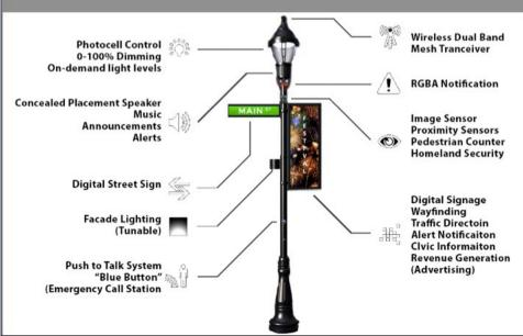
An important first layer of smart city technology is the public streetlight, which can support multiple functions on a single piece of equipment. Products like these are fully available today, even if the network and data infrastructure behind them isn't yet fully deployed in most cities.
