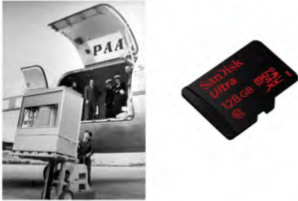
The IBM Model 350 disk file with a storage space of 5MB from 1956 and a Micro SD Card
